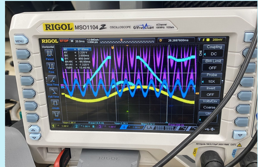
Two's Complement error on visualized with oscilloscope
