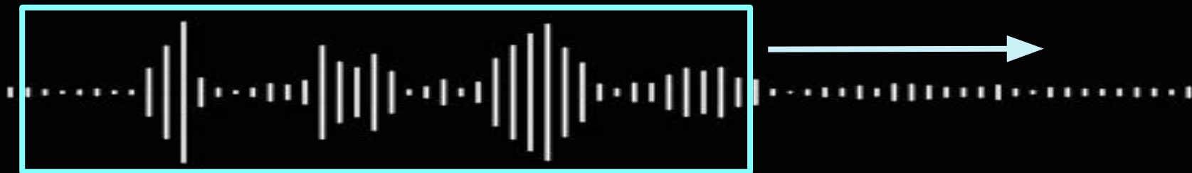
A sliding window of 128 samples is used to manipulate audio
